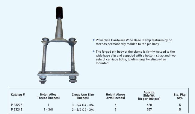
Also available in Lead Thread; Remove Z to Part Number if lead is required
